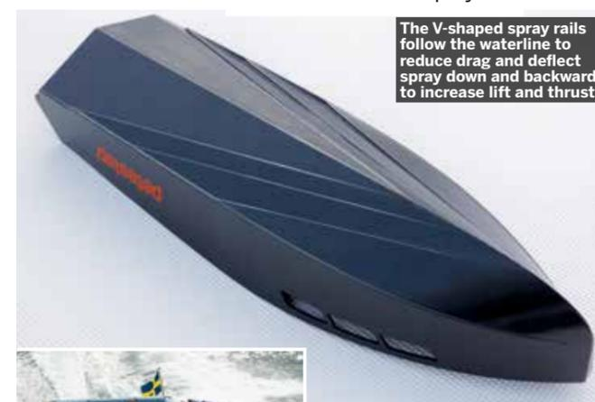
The V-shaped spray rails follow the waterline to reduce drag and deflect spray down and backwards to increase lift and thrust
